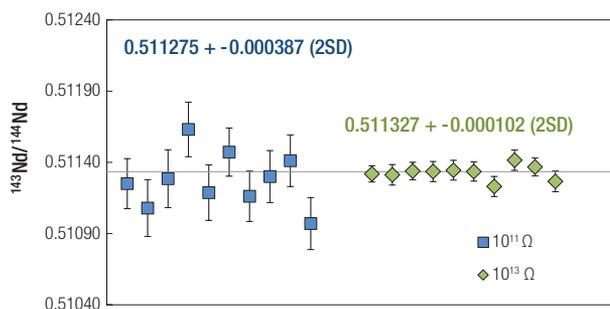
Figure 6. External reproducibility for  $^{143}\text{Nd}/^{144}\text{Nd}$  isotope ratios measured on  $10^{11} \Omega$  and  $10^{13} \Omega$  amplifiers.
