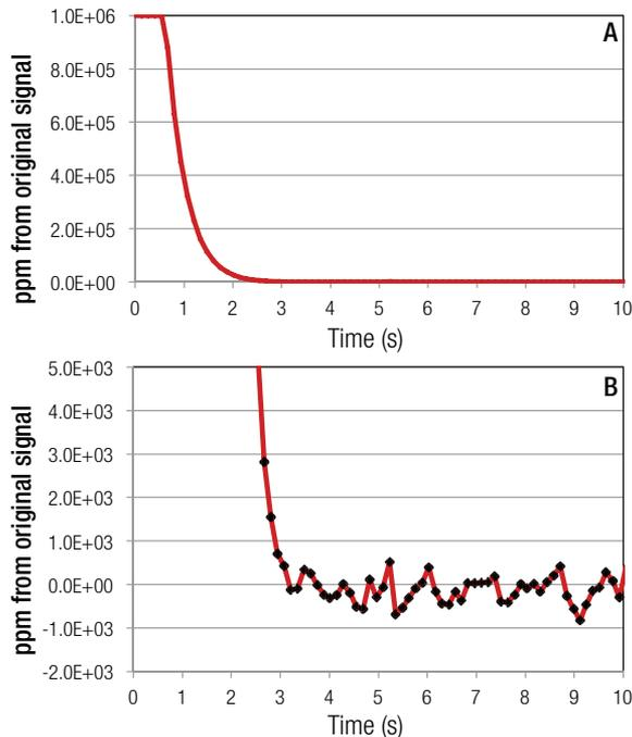
Figure 3. a) Typical signal decay for a  $10^{13} \Omega$  amplifier, b) same, but with adjusted y-axis scale (zoom-in).
