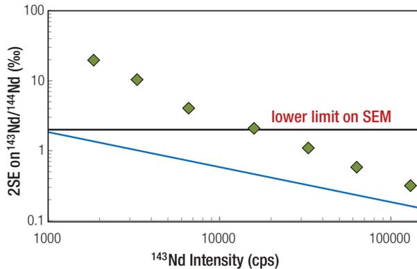
Figure 8. Comparison of the internal precision of  $^{143}\text{Nd}/^{144}\text{Nd}$  on SEM vs  $10^{13}\ \Omega$  amplifiers.
