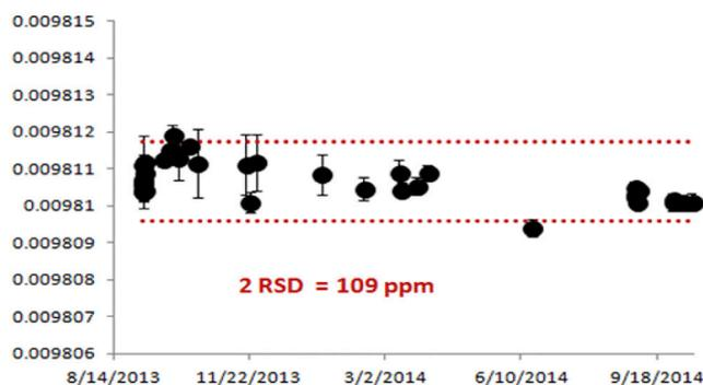
Figure 4. Long-term gain stability of a  $10^{13} \Omega$  amplifier.
