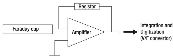
Figure 1. Schematic representation of the Faraday cup detection system. The Faraday cup is connected to electrical ground via an amplifier that is equipped with a high ohmic resistor. The amplified signal is converted to volts by a V/F converter.  $V = I \times R$ , where  $V$  = voltage;  $I$  = ion current;  $R$  = resistivity. Current amplifiers can be equipped with resistors with  $R = 10^{10}$ ,  $10^{11}$ ,  $10^{12}$  or  $10^{13} \Omega$ .
