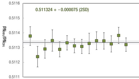
Figure 7. External reproducibility of  $^{143}\text{Nd}/^{144}\text{Nd}$  on individual 100 pg Nd loads using  $10^{13}\ \Omega$  amplifiers.
