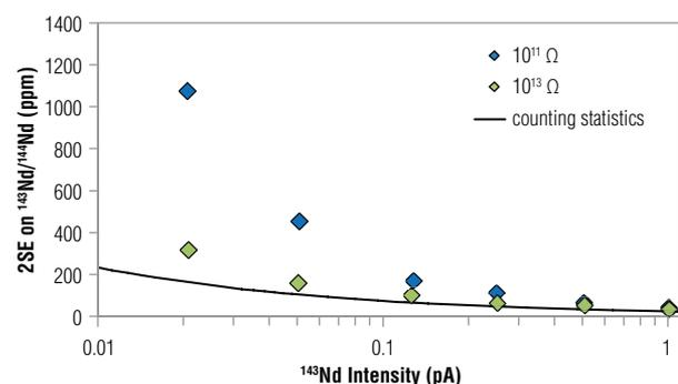
Figure 5. Internal precision on  $^{143}\text{Nd}/^{144}\text{Nd}$  as function of ion beam intensity using  $10^{11} \Omega$  and  $10^{13} \Omega$  amplifiers.
