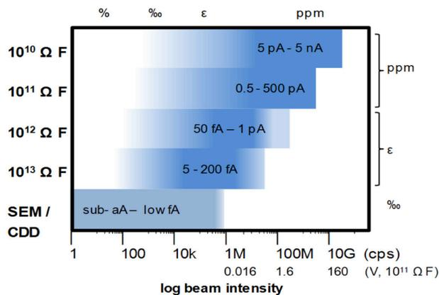
Figure 9. Dynamic range of different detector types (F = Faradays Cup).
