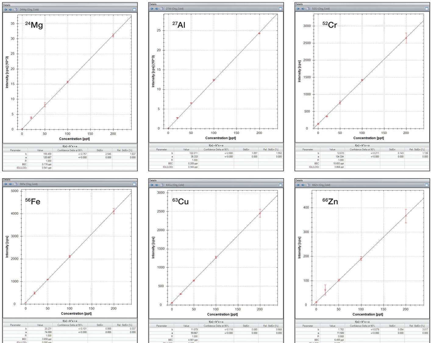
Figure 3. Cold plasma calibration curves with points 20, 50, 100 and 200 (ng·L<sup>-1</sup>).
