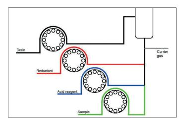
Figure 2. Schematic of the VP100 vapor generation accessory showing how the sample, acid and reductant are mixed.
