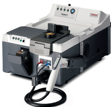
Figure 2. Thermo Scientific Antaris II MDS system. This system includes a transmission cell used for analyzing liquids such as the beer samples used in the present application.
