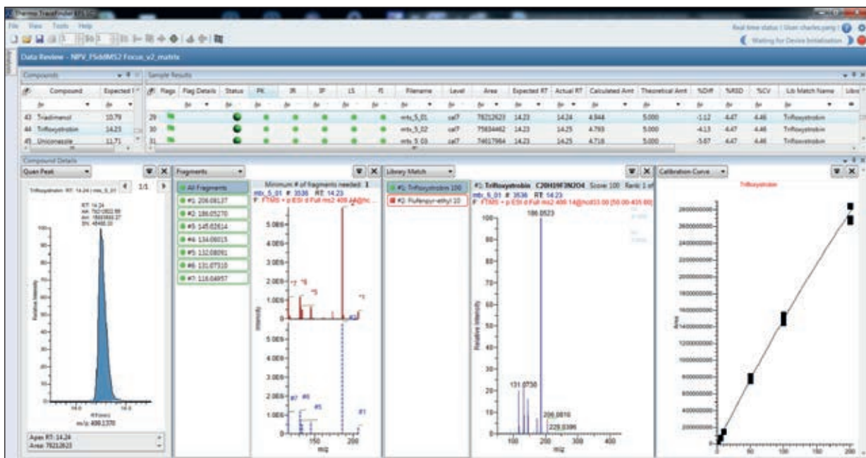
Figure 5. Tryfloxystrobin at 5 ppb, showing compound details in lower portion to highlight quick data review.
