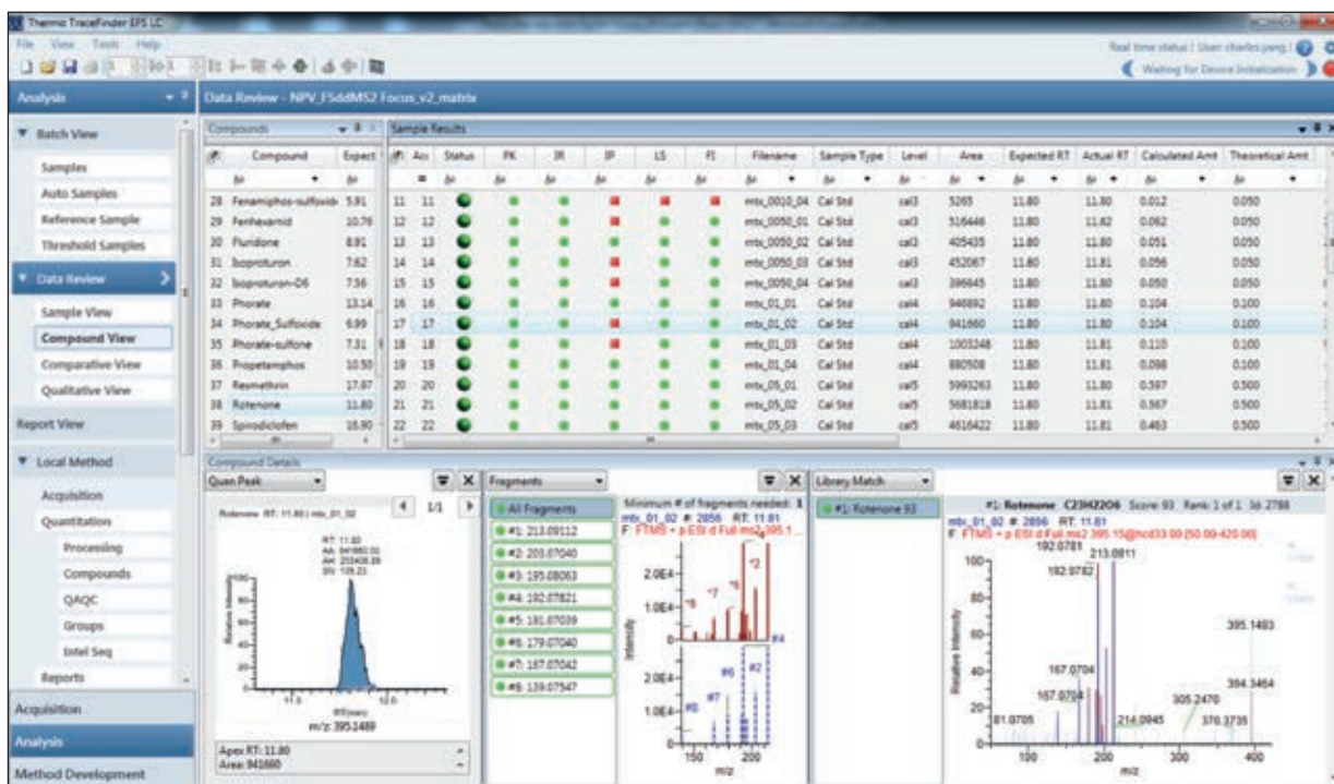
Figure 13. Rotenone library match confirmation with fragmentation confirmation at 1 ppb, showing a library match score of 93% confidence in the lower right pane.
