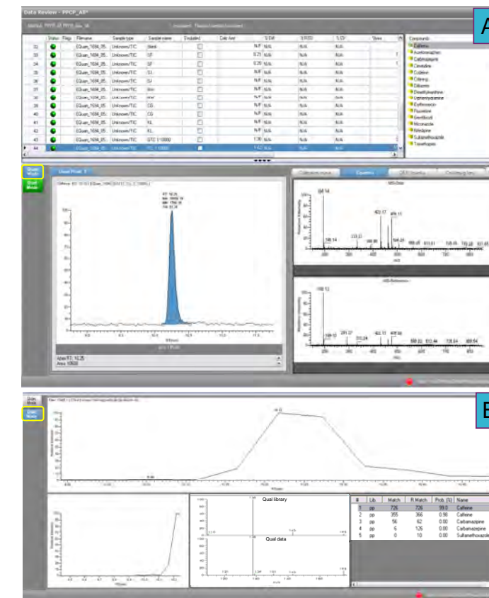
FIGURE 7. Panel A depicts the quantitative results for the Iced Tea Lemon samples full scan data and reference spectrum. Panel B depicts the automated confirmation results (Qual mode) showing the NIST library search results.
