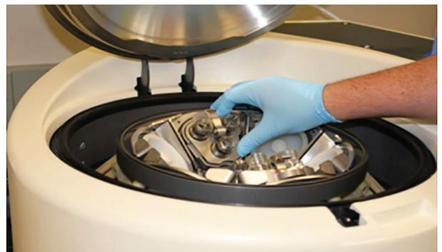
Figure 4. Dionex ASE Pucks are loaded into the Rocket Evaporator.
