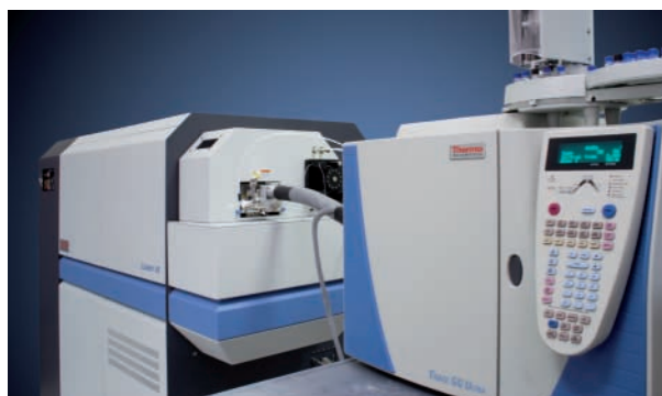
Figure 1: Thermo Scientific TRACE GC Ultra coupled to the Thermo Scientific ELEMENT 2 HR-ICP-MS.
