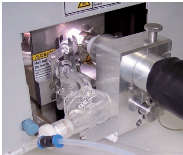
Figure 2: Dual Sample Introduction System.
