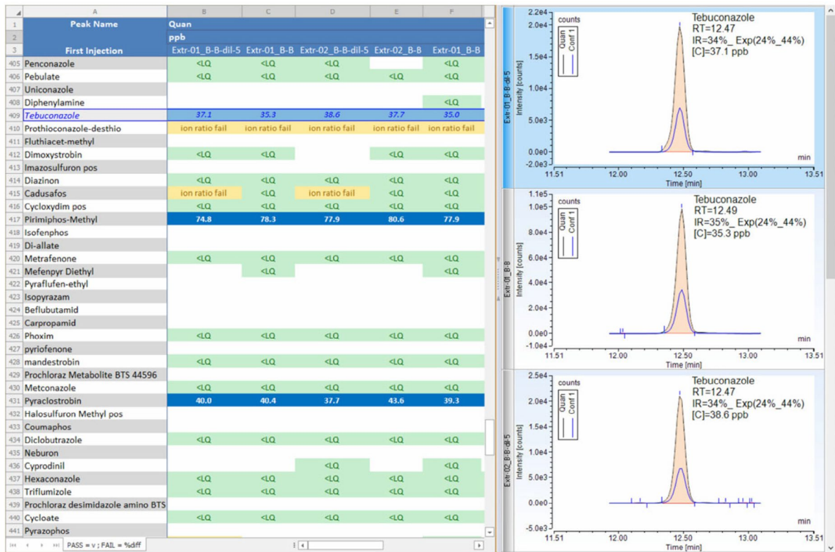
Figure 7. Data review: Ion Ratio check and calculated amount for samples. This view allows quick confirmation that ion ratios are in the expected range and provides sample results.
