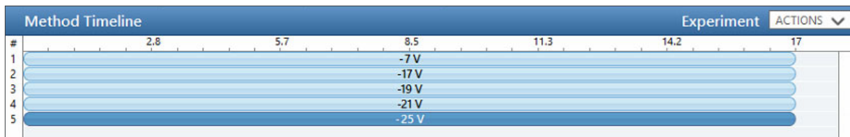
Figure 4. Method used for sulfonamide analysis that includes five parallel experiments differing only in the CV value
