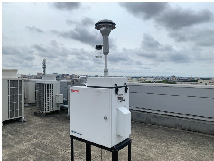
Figure 1. Sample collection at Kanagawa prefecture (location 1) using the Partisol 2025i system
