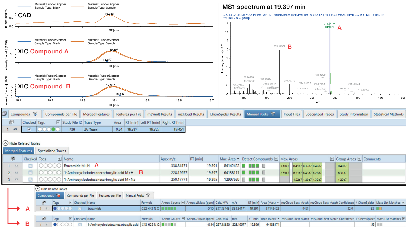
Figure 7. Correlation of CAD peak at 19.38 min with MS compounds with monoisotopic molecular weight of 337.3344 Da ( C_{22}H_{43}NO , erucamide, identified based on MS/MS spectral match) and 227.1885 Da ( C_{13}H_{25}NO_2 , 1-aminocyclododecanecarboxylic acid, putative annotation based on mzLogic ranking of mass list and ChemSpider matches) with their XICs and MS1 spectrum shown
