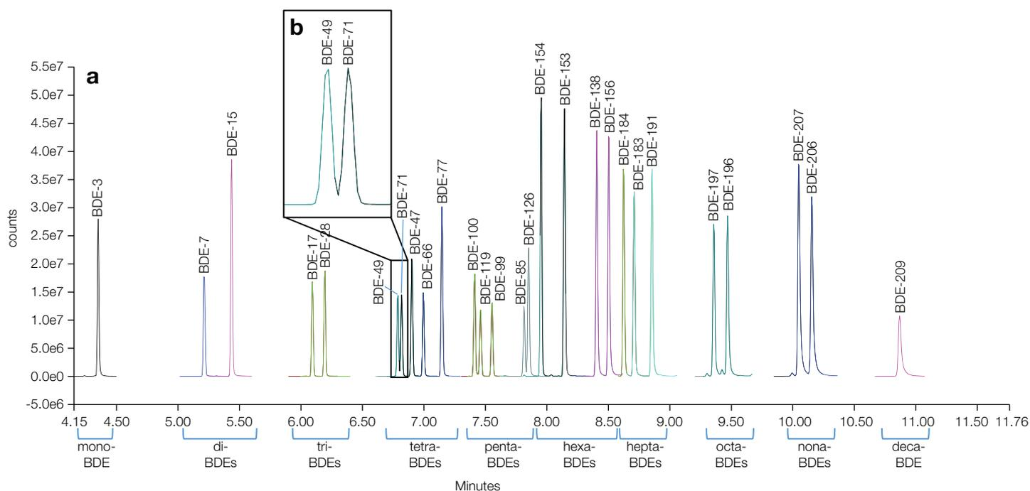
Figure 3. (a) Overlaid extracted ion chromatograms (EICs  $\pm 5$  ppm extraction window) for the 27 native PBDE congeners in a solvent standard at 400 pg on column for mono- to penta-BDEs, 800 pg on column for hexa- to octa-BDEs, and 2000 pg on column for nona- to deca-BDEs and (b) separation of critical pair (BDE-49 and BDE-71)
