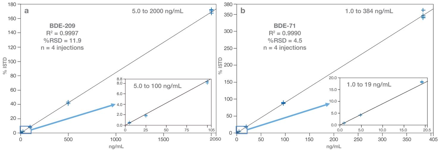
Figure 8. Example calibration curves (a) BDE-209 and (b) BDE-71, illustrating the linearity obtained. The inset calibration curves exemplify the maintained linearity for the lowest 3 calibration levels.
