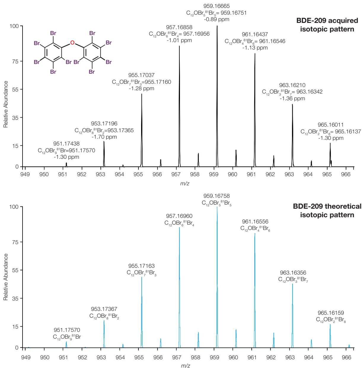
**Figure 5. Comparison of mass spectra for BDE-209, acquired isotopic pattern (upper) versus the theoretical isotopic pattern (lower).** Consistent <2 ppm mass accuracy obtained for each of the ion in the cluster. Annotated are the measured mass, the elemental composition, and the theoretical mass as well as the mass accuracy (ppm).
