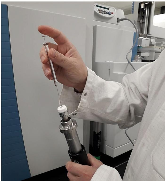
Figure 1. DIP sample loading procedure
