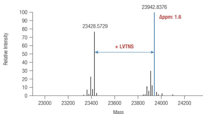
**Figure 5. Deconvoluted mass spectrum of trastuzumab biosimilar light chain region.** An intense signal at 23942.8376 Da is visible; this corresponds to the addition of five amino acids belonging to the signal peptide only partially cleaved from the antibody. Accurate mass ( $\Delta < 2$  ppm) allowed the unambiguous identification of this variant.
