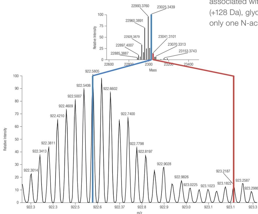
**Figure 3. Light chain analysis of rituximab drug product.** The MS and deconvoluted spectra show the peaks processed to obtain light chain (red) and light chain modified at position Q1 with a pyroglutamic acid (blue).
