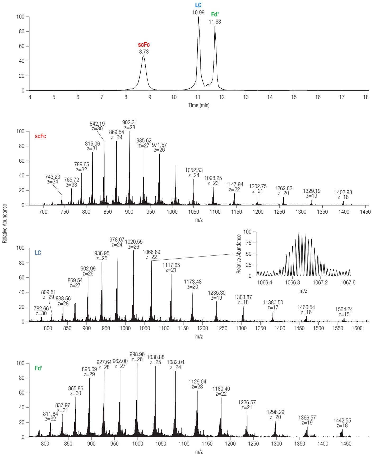
**Figure 2.** LC-MS analysis of IdeS digested bevacizumab biosimilar. In the top panel the TIC trace shows the three subunits obtained after enzymatic digestion and separated on a MabPac RP, 2.1 × 50 mm column. Bottom panels show the charge envelope profiles obtained for the three subunits using the protein mode on the Q Exactive Plus mass spectrometer; in the zoom it is possible to observe fully isotopically resolved peaks for +22 charge state of the LC region.
