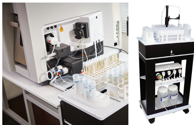
Figure 2. prepFAST Autodilution system connected to the iCAP RQ ICP-MS (left). ESI SC-2DX Autosampler (right).
