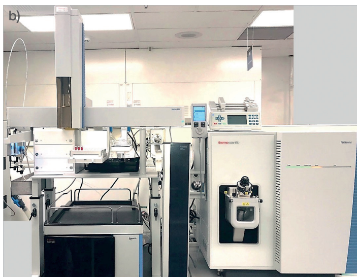
Figure 1. TriPlus RSH with \mu SPE capabilities system: a) TriPlus RSH modules required to perform the \mu SPE clean-up procedure and b) coupled to LC-MS/MS
