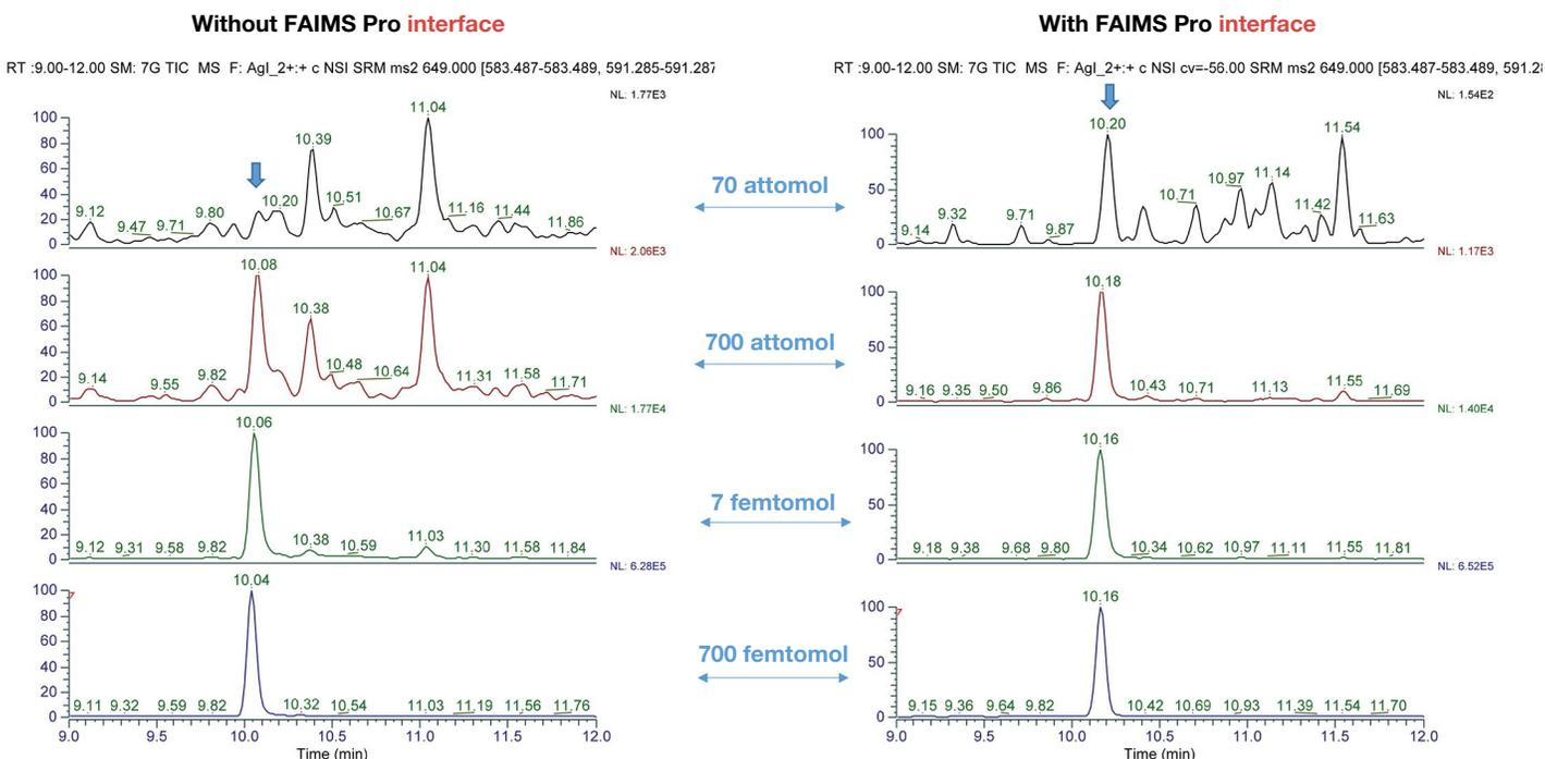
**Figure 4. Quantification of angiotensin I in digested plasma.** Combining the FAIMS Pro interface with an optimized CV value as part of the SRM table provides selective noise reduction, which results in a quantifiable signal (right panels) even at concentration levels where analyte signal is impacted by noise interference without FAIMS Pro interface (left panels).
