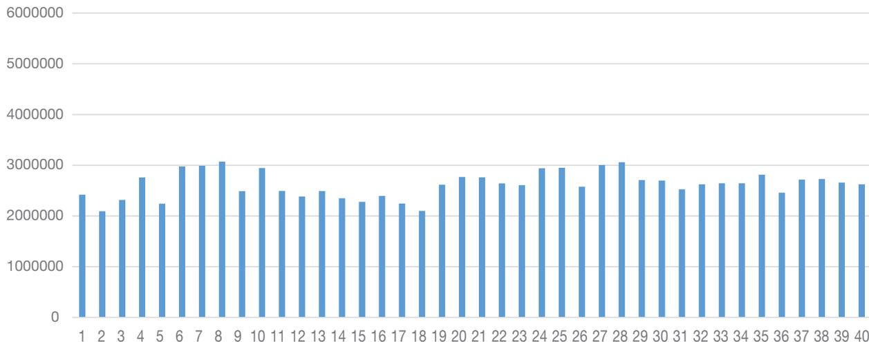
**Figure 5. 40 consecutive injections of angiotensin I in 0.5  $\mu\text{g}/\mu\text{L}$  digested plasma were performed with the FAIMS Pro device on the TSQ Altis triple quadrupole mass spectrometer.** The overall % RSD was <10% across a 2-day experiment. (Thermo Fisher™ ChromaCare™ solution was injected every 10 analytical injections for column clean-up.)
