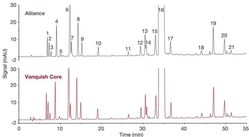
**Figure 1. Transfer from Alliance system to Vanquish Core HPLC system according to the EP monograph for chlorhexidine gluconate; peak assignment according to impurity designation in EP monograph and standard leaflet<sup>5,9</sup>**
