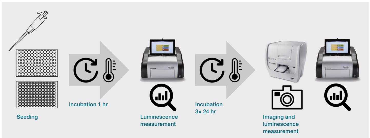
**Figure 1. Procedure to assess viability and morphology of the cells.** Seeding of the cells in 96-well and 384-well plates, incubation and analyzing steps during 72 hours.\*
