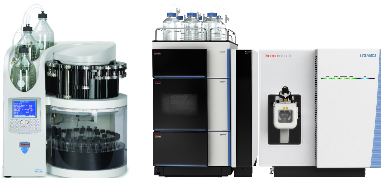
Figure 1. Dionex ASE 350 accelerated solvent extractor (left) and TSQ Fortis triple-quadrupole mass spectrometer (right)
