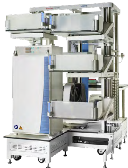
Figure 2: The Thermo Scientific™ inSPIRE™ platform integrated with various instruments including the Thermo Scientific™ Cytomat™ Automated Incubator Series. These instruments are placed on tables, platforms, and shelves integrated around the central frame containing the Thermo Scientific™ Spinnaker™ XT Microplate Robot and controlled by the Thermo Scientific™ Momentum™ Workflow Scheduling Software.
