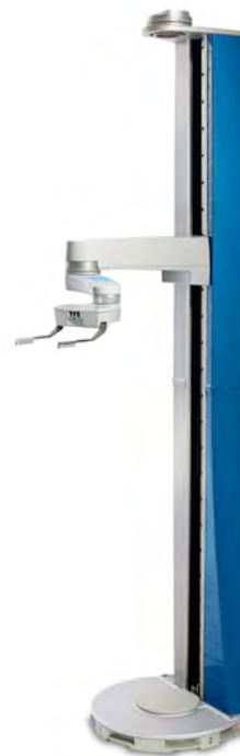
Figure 4: The Thermo Scientific™ Spinnaker™ XT robot is the central mover to the inSPIRE platform, and it is responsible for microplate transportation between all instruments on the system.
