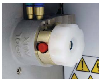
Figure 4: EMT torch for ease of use for routine maintenance.
