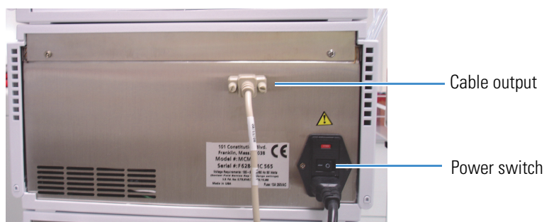
Figure 132. The null modem cable attaching the MCM to the TLX system
