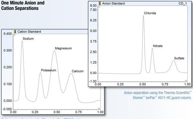
Cation separation using the Dionex IonPac CS12A column.
