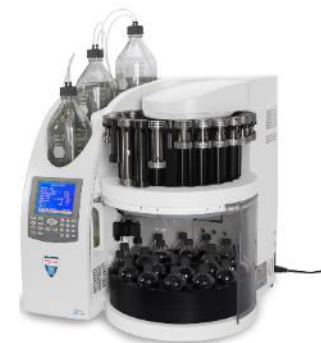
Accelerated solvent extraction technique (30 minutes)
