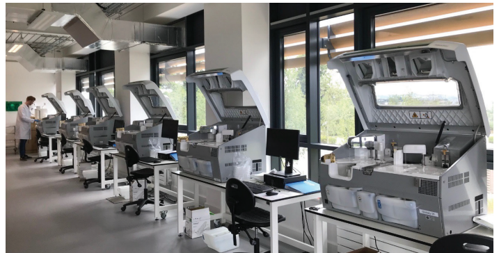
Several Thermo Scientific™ Gallery™ Plus Discrete Analyzers are in operation providing high-throughput wastewater biomarker analysis at the NLS's Exeter laboratory. Photo courtesy of the NLS.
