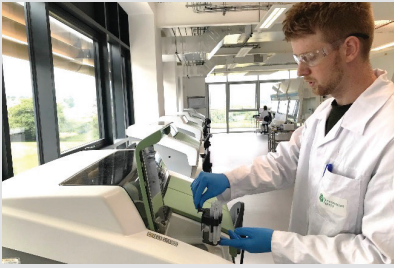
An NLS analyst loads wastewater samples into a Gallery Plus discrete analyzer. Photo courtesy of the NLS.
