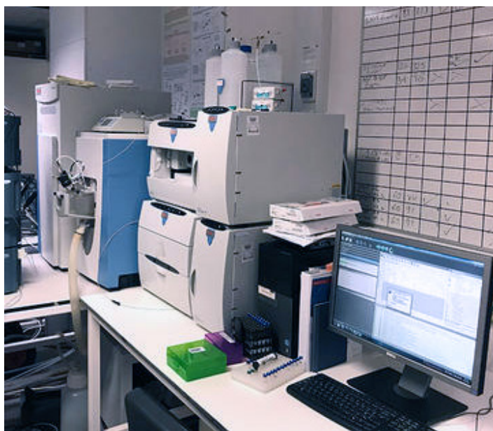
Thermo Scientific™ Dionex™ ICS-5000+ Ion Chromatography System with the Thermo Scientific™ Q Exactive™ Hybrid Quadrupole-Orbitrap Mass Spectrometer advances metabolomics research. Photo courtesy of the Mass Spectrometry Research Facility (SRF), Chemistry Research Laboratory, University of Oxford.
