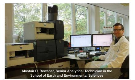
Alastair D. Bewsher is a Senior Analytical Technician in the School of Earth and Environmental Sciences. He uses a Thermo Scientific<sup>™</sup> Dionex<sup>™</sup> Capillary HPIC<sup>™</sup> system equipped with **Thermo Scientific<sup>™</sup> Dionex<sup>™</sup> IonPac<sup>™</sup> AS11-HC-4µm IC columns** for analyzing anions and organic acids.
