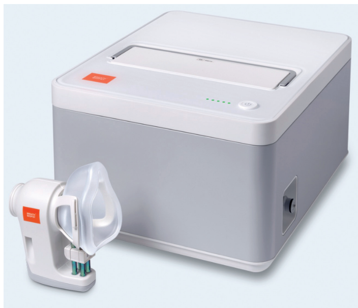
Figure 4. The ReCIVA Breath Sampler (left) enables reliable, reproducible collection of breath VOCs and pre-concentration for enhanced sensitivity. Pressure and CO 2 sensors in ReCIVA provide real-time monitoring of the subjects breathing, allowing different breath fractions to be sampled in a single collection event if desired. ReCIVA works in partnership with the CASPER Portable Air Supply (right) that filters air prior to inhalation to remove background VOCs.
