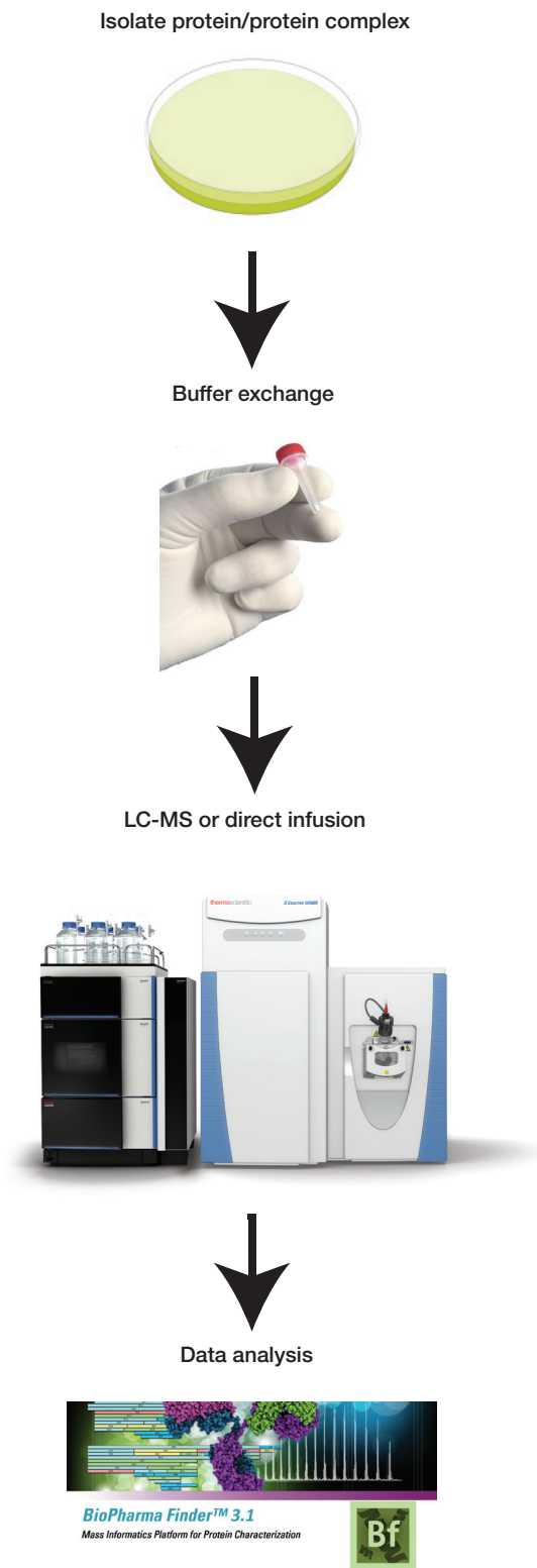
Figure 4. Schematic representation of a typical native MS workflow
