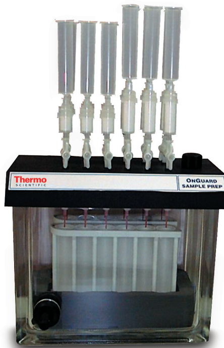
Figure 7. Samples can be processed in parallel using the Dionex OnGuard Sample Prep Station.
