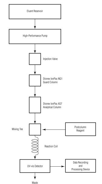
Figure 3. System flow diagram.
