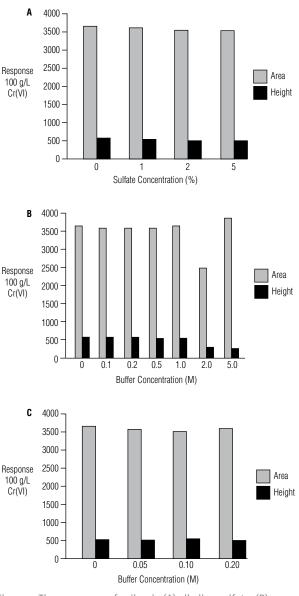
Figure 5. The responses of spikes in (A) alkaline sulfate, (B) acetate buffer, and (C) carbonate buffer samples.
