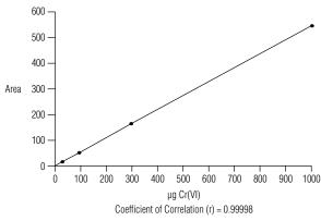
Figure 4. Area response for colorimetric chromium detection.
