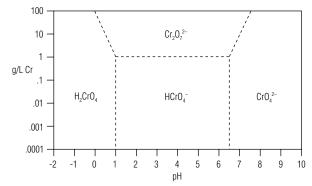
Figure 1. Relative distribution of Cr(VI) species in water as a function of pH and Cr(VI) concentration.
