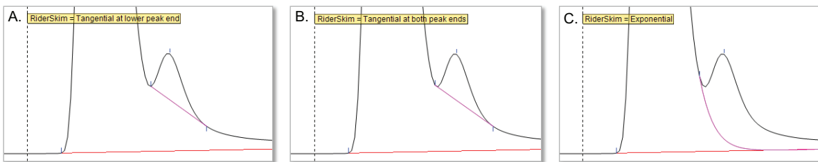
Figure 43. A: Tangential at lower peak end, B: Tangential at both peak ends, C: Exponential.
