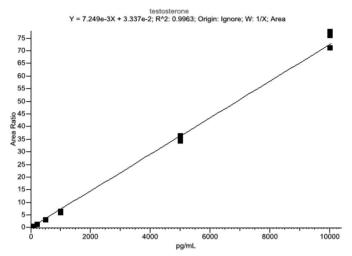
Figure 2. Calibration curve for testosterone (5-10,000 pg/mL)
