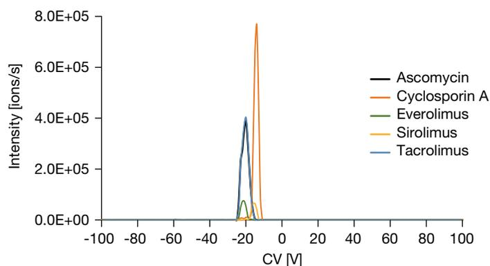
**Figure 1. Optimization of CVs for immunosuppressants that identified final settings of -14 V for Cyclosporin A, -16 V for Sirolimus, and -21 V for Tacrolimus, Ascomycin, and Everolimus**
