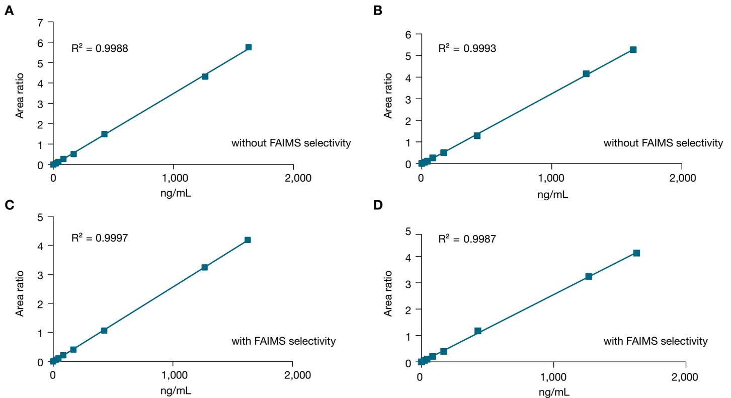
Figure 5. Comparative quantitation curves for Cyclosporin A in crashed whole human blood. Area under the curve ratios were determined as compared to the internal standard Ascomycin. Quantitation curves 5A and 5B were acquired without FAIMS selectivity on days 1 and 5, respectively, and curves 5C and 5D were acquired with FAIMS selectivity on days 1 and 5.
