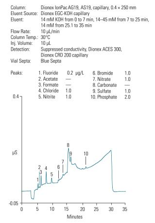
Figure 8. A large-loop direct injection of a 1:100,000 diluted Dionex Seven Anion II Standard onto a capillary Dionex IonPac AS19 column set.A) 2 mm microbore and B) 0.4 mm capillary columns.
