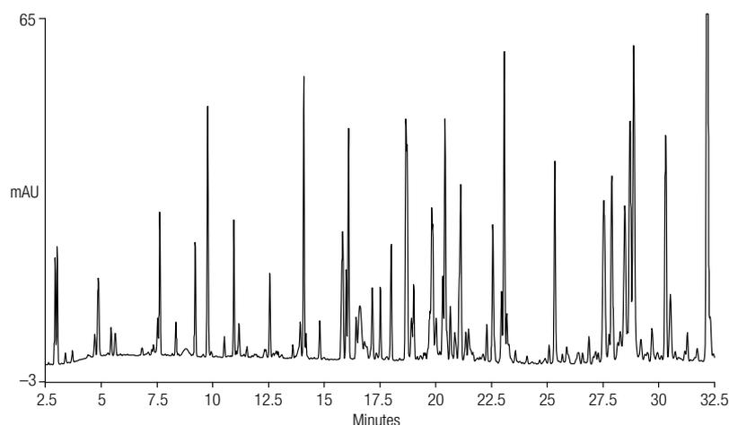
Figure 2. Separation of mAb 10mg/mL tryptic digest at 80 °C and 30 min gradient. Injection volume 1  $\mu$ L. Pump module: DGP-3600RS.
