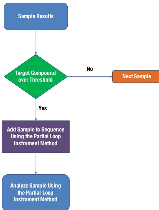
Figure 1. Flow chart of the Chromeleon 7 CDS AutoDilution process.
