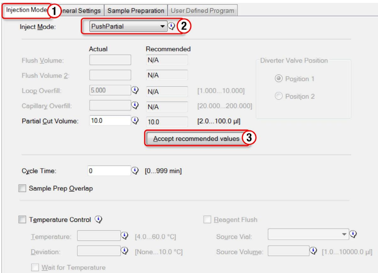
Figure 2. Configuring the Partial Injection mode of the Dionex AS-AP autosampler.
