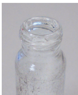
Figure 2b. Typical re-wash screw thread damage
