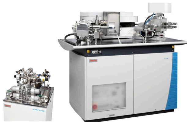
Figure 1. Thermo Scientific Helix MC Plus Noble Gas MS (right) and NG Prep System (left).
