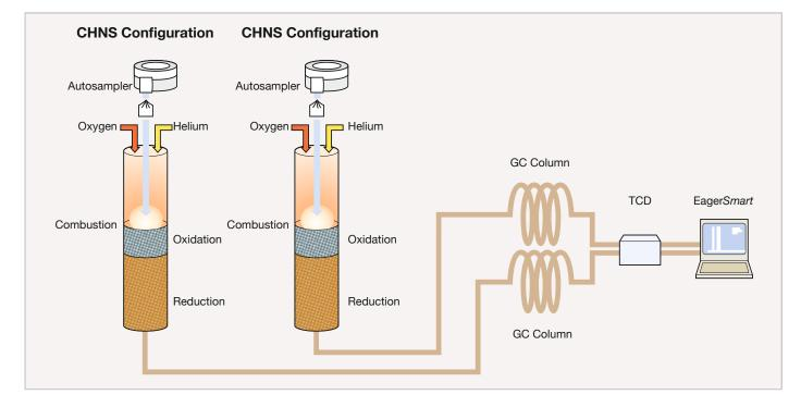
Figure 3. FlashSmart CHNS/CHNS configuration.
