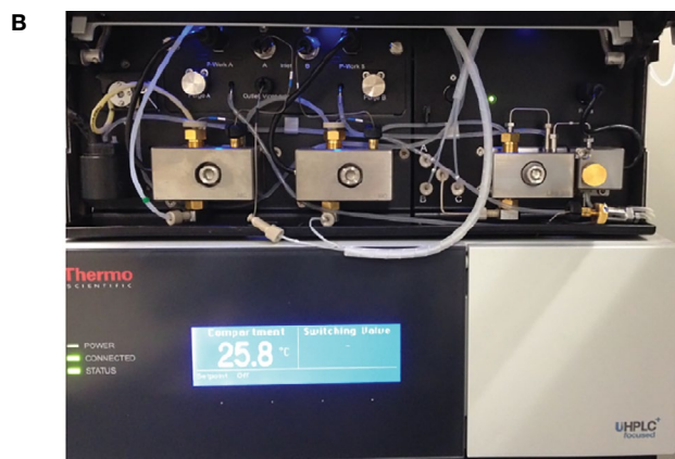
Figure 2. (A) HDX workstation sample delivery path: cooling chamber; (B) UltiMate NCS-3500RS LC system with binary rapid separation micro flow pump and quaternary loading pump
