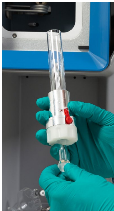
Figure 2. iCAP PRO Series ICP-OES EMT Torch
