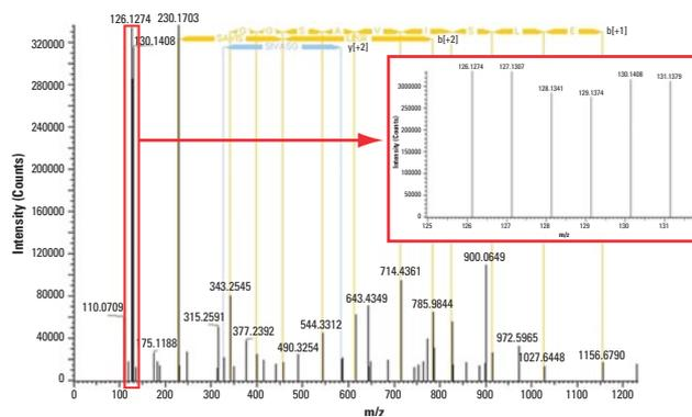
**Analysis of a TMTsixplex-labeled peptide by pulsed Q dissociation (PQD) and high energy collision dissociation (HCD).** TMTsixplex-labeled A♦ITIFQER (2+) from rabbit glyceraldehyde-3-phosphate dehydrogenase in a 10-protein sample were mixed at a 1:2:3:4:2:0.5 ratio. Shown are the MS/MS spectra for the peptide fragment and reporter ion regions. PQD fragmentation was performed on a Thermo Scientific LTQ XL Ion Trap and by HCD on a high-resolution Orbitrap XL Mass Spectrometer.
