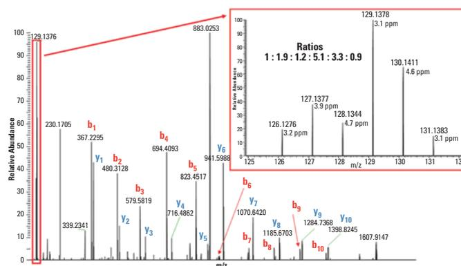
**Analysis of a TMTsixplex-labeled mix of bovine serum albumin on a high-resolution Thermo Scientific Orbitrap XL Mass Spectrometer.** MS/MS fragment ions in the peptide fragmentation and reporter ion regions for the ◆HLVDEPQNLIK◆ (+2) peptide. BSA tryptic digests were labeled with TMT<sup>6</sup> Label Reagents and mixed at a 1:2:1:5:3:1 ratio.
