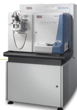
Orbitrap Velos Pro Hybrid Ion Trap-Orbitrap Mass Spectrometer
