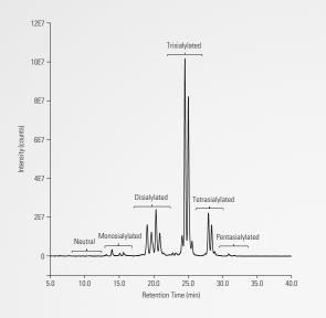
The GlycanPac AXR-1 column is based on novel mixed-mode column chemistry, combining the retention mechanisms of both WAX and reversed-phase (RP) properties for optimal selectivity and resolution. The WAX functionality provides retention and selectivity for negatively charged glycans, while the reversed-phase mode facilitates the separation of glycans of the same
