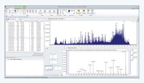
Mass Frontier software extracts the multiple components that can occur underneath chromatographic peaks. Each blue triangle is a detected component.
