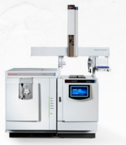
Thermo Scientific Orbitrap Exploris GC mass spectrometer
