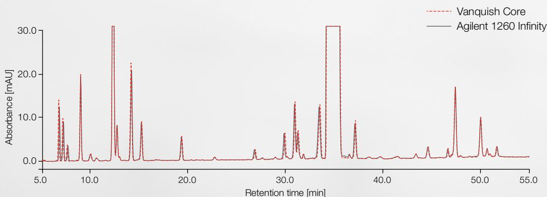
**With the Vanquish Core HPLC system, the instrument gradient delay volume can be seamlessly adjusted in order to match legacy HPLC instruments. In this example the gradient delay volume was increased by a simple software command (Idle Volume=200  $\mu$ L) in the instrument method to best match the Agilent® 1260 Infinity LC system.**
