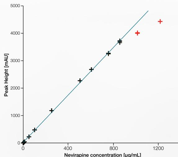
Concentration vs. peak height plot of nevirapine with data points that were considered for calibration (black) and data points that were eliminated from calibration due to curve decline (red). Linear calibration with permitted offset and no weighting.
