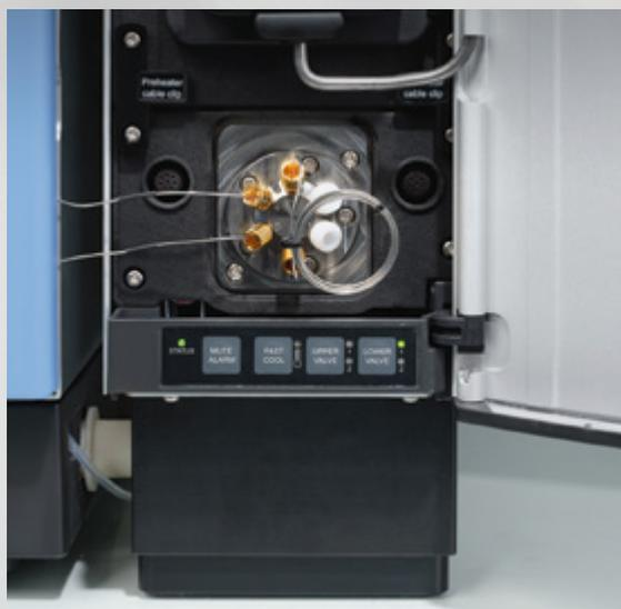
Method Transfer kit for Vanquish Core HPLC system. In combination with the Vanquish Split Samplers metering device, the gradient delay volume can be adjusted on a microliter scale over a wide range. Audit trail tracking of the settings and full qualification ensure regulatory compliance.
