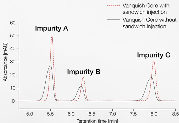
High organic sample solvents can cause peak shape distortions on modern HPLC instruments. Vanquish Core HPLC systems conduct sandwich injections to be able to inject high organic samples while keeping the chromatographic efficiency.
