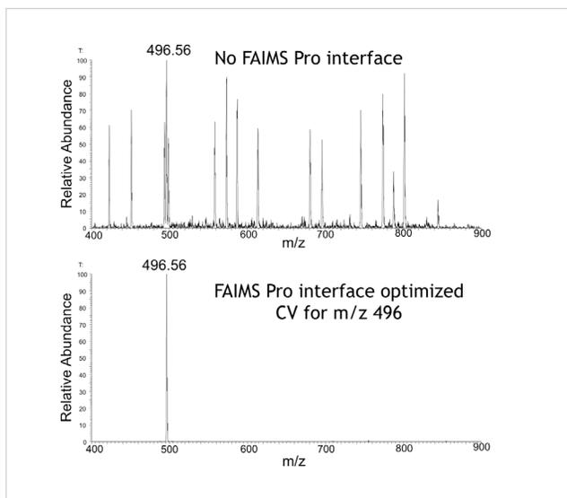
Figure 2. Gas phase separation provides an additional level of selectivity for precursors. The result is a reduction in isolation interference, even without chromatographic separation. Here the compensation voltage (CV) was optimized for transmission of precursor  $m/z$  496, selectively enriching for this target. Data collected on a Orbitrap Eclipse Tribrid MS.
