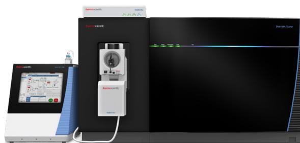
Thermo Scientific™ EASY-nLC™ 1200 system and FAIMS Pro interface coupled to the Orbitrap Eclipse Tribrid MS.
