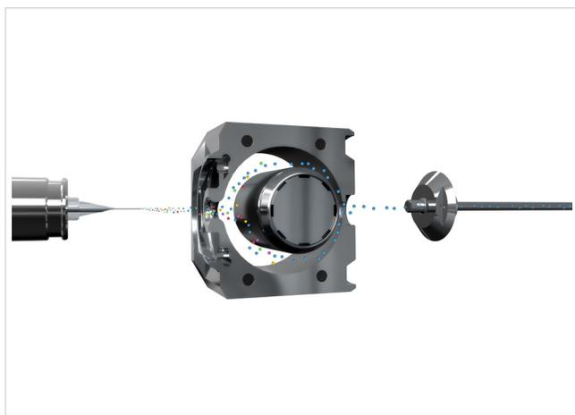
*Figure 1. High field asymmetric ion mobility spectrometry (FAIMS) spatially separates ions between strong and weak electric fields. Ions (multi-colored) transverse the interface between the cylindrical electrodes based upon differences in the ion mobility. Only ions with a stable flight path (blue) enter the mass spectrometer. Therefore FAIMS increases selectivity and enables gas-phase fractionation.*
